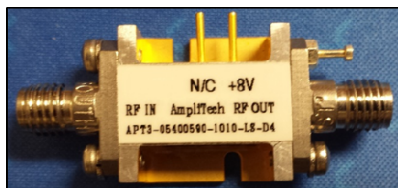
C-Band Super Low Noise Amplifier with integrated 2W CW Limiter
