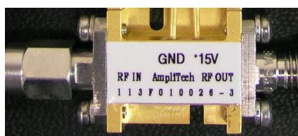
C-Band Super LNA/High Dynamic Range with integrated Bias- Tee
