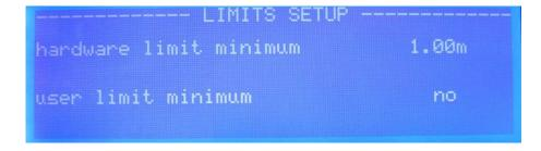
You can type in a user limit and confirm with "ENTER". To delete the user limit type in a value lower then 1, e.g. 0, and confirm with "ENTER". Press "EXIT" and you will be back in the MAINSCREEN.
