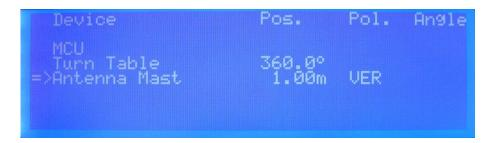
You will be able to change the polarization and to move up and down manually or with entering a new height.
