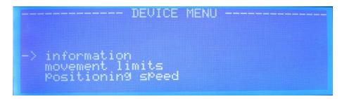
2. Navigate to "information" and press "ENTER". The device type, the serial number and the firmware version is shown.
