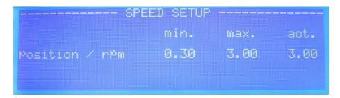
You can change the actual speed by type in a value and confirm with "ENTER". Press "EXIT" to go back to the MAINSCREEN.
