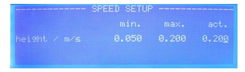
You can change the actual speed by type in a value and confirm with "ENTER". Press "EXIT" to go back to the MAINSCREEN.
