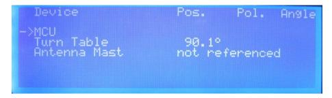
In this example the main screen shows the MCU itself, a referenced Turntable and a non-referenced Antenna Mast.
