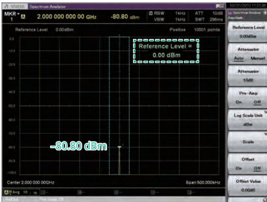
Example: Level Stability by Switching Reference Level
