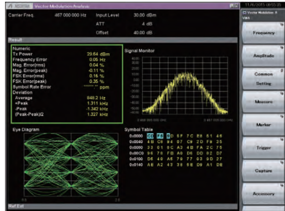
4FSK Modulation Analysis Measurement Example
