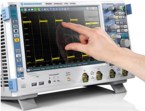
High-resolution capacitive touchscreen allows users to perform functions through gestures.
