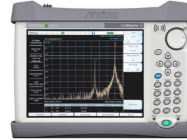
Cable and Antenna Analyzers with integrated Spectrum Analyzer
