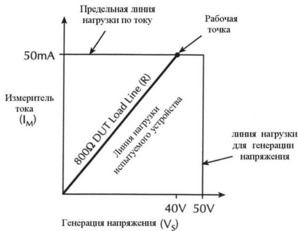
$$\begin{aligned} V_S &= I_M \cdot R \\ &= (50mA) (800\Omega) \\ &= 40V \end{aligned}$$
