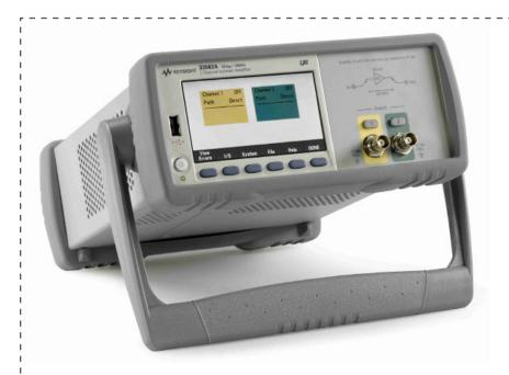
The Keysight 33502A is a dual-channel, high voltage output amplifier. It has an isolated analog front end with up to 50 Vpp (± 25 V) output voltage range. It is also a very low-distortion amplifier with < 0.01% @ 10 kHz and 40 Vpp. The 33502A is designed to work as a companion for function generators to offer low-distortion, higher voltage outputs.
