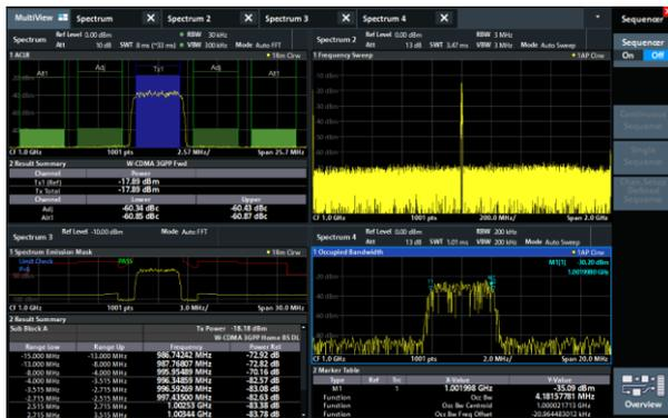
Configure your result windows the way you want. Display different measurement channels at once. Sequential channel updating allows parallel measurement of e.g. spectrum, spectrogram, I/Q analysis and analog demodulation.
