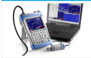
The R&S°FSH can be remotely controlled via the USB or LAN interface and integrated into user-specific programs.
