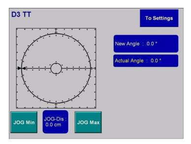
By pressing key for Antenna Mast the picture below appears and the antenna mast is activated. Masts must be referenced before positioning is enabled. By pressing "To Settings" the adjustment possibilities for the device are shown.
