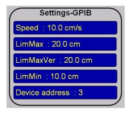
At this menu the speed with GPIB or LAN, the relevant limits and the device addresses are indicated.
