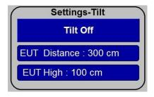
At this menu it is possible to activate or deactivate the tilt function and to set the measurement distance and EUT height.
