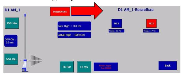
If an error appears regularly or always, you can get additional information to the error by pressing "NC1" – "NC4" Buttons. Each single motor of the device has its own NC menu. The screen below appears and provides more detailed information. This can be important for maturo to give a quick solution to your problem.
