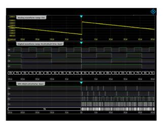
With the R&S\*RTE-B1 option, every R&S\*RTE can be turned into particle a mixed signal oscilloscope with 16 digital channels. This example shows the ramp signal of a 4-bit ADC with analog and digital channels correlated to an SPI bus that controls the ADC.
