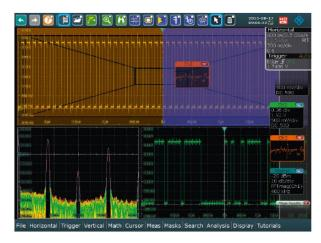
You can drag & drop waveforms and result windows on the screen. The SmartGrid function helps you flexibly arrange multiple diagrams on the screen.
