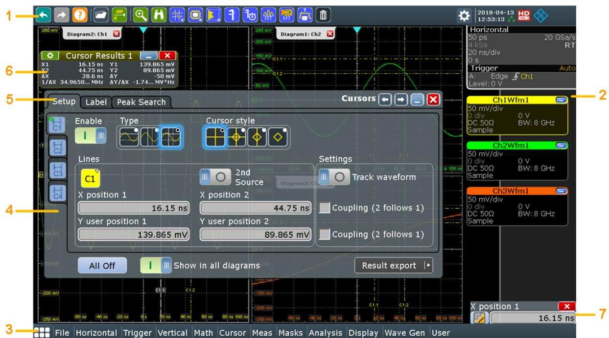
**Figure 5-4: Control elements on the touchscreen**
