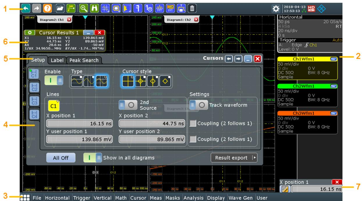
**Figure 5-4: Control elements on the touchscreen**
