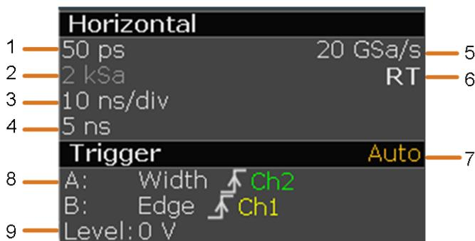
**Figure 5-2: Horizontal and trigger label on top of the sidebar**
