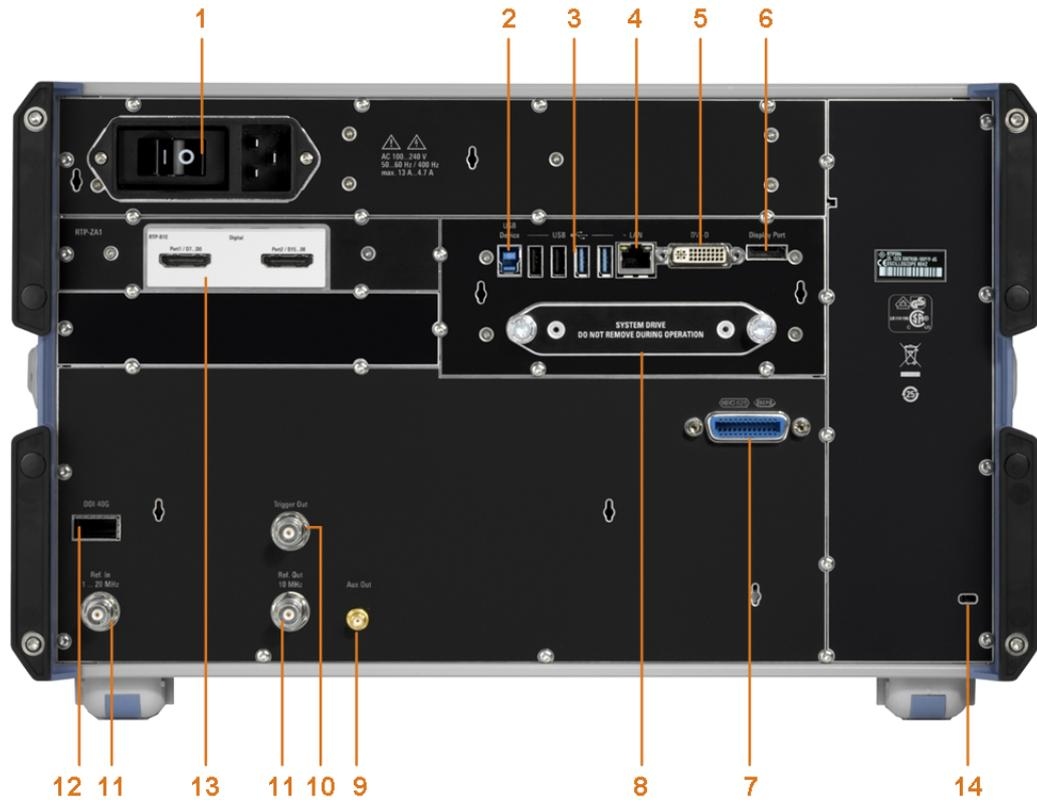
**Figure 4-2: Rear panel of R&S RTP**
