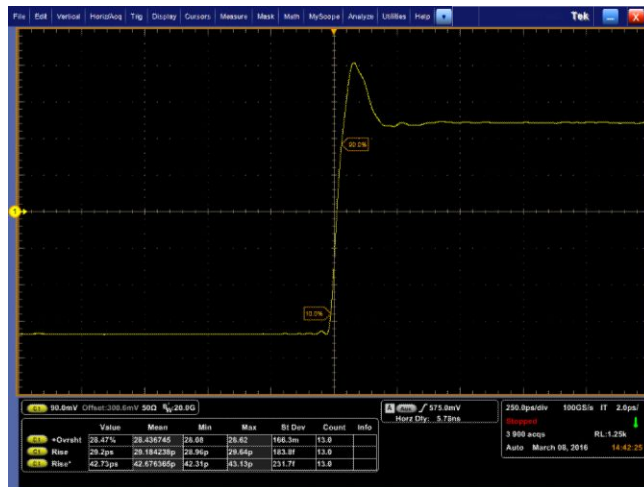
Figure 20: P77STFLXA solder tip attached with 300 mils (7.62 mm) wires (rise time = 42.8 ps)
