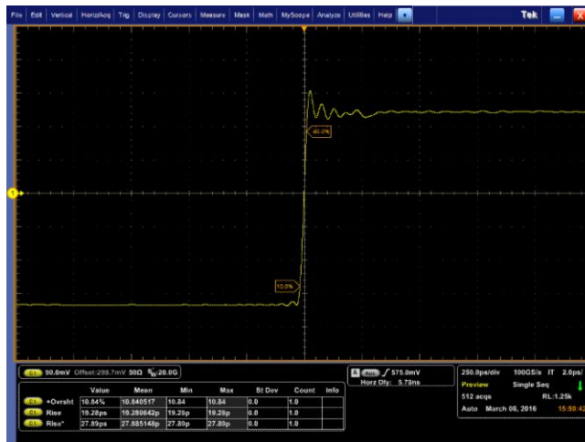
Figure 17: P77STFLXA solder tip attached with 75 mils (1.90 mm) wires (rise time = 27.9 ps)
