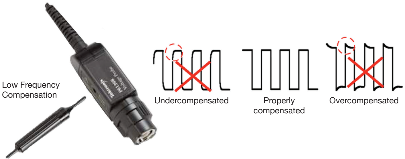
Figure 4. Low Frequency Probe Compensation.
