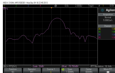
Spectrum signal comparison. (CF 900 MHz; span1 MHz; RBW 1 kHz (MDO3104), 19.1 kHz(X3104A)). MDO3000 also offers automatic markers and spectrogram display.
