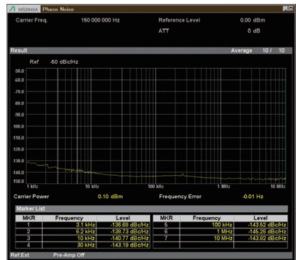
Phase Noise Measurement Low Phase Noise Performance MS2840A-066 On 150 MHz Measurement Frequency, Preamp Off
