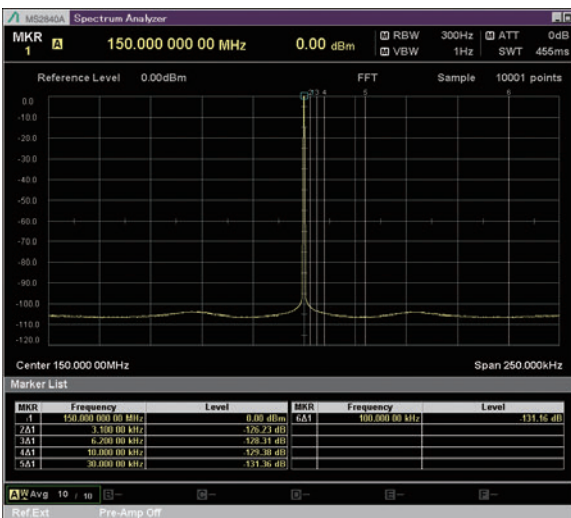
Spectrum Display Low Phase Noise Performance MS2840A-066 Off 150 MHz Measurement Frequency, Preamp Off
