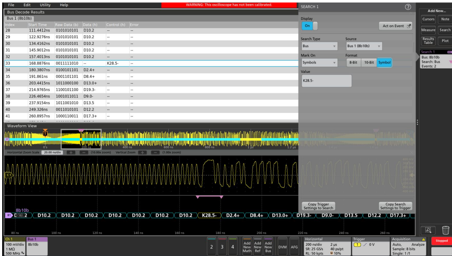
Searching on a specific data symbol in symbol format on a 8b10b bus
