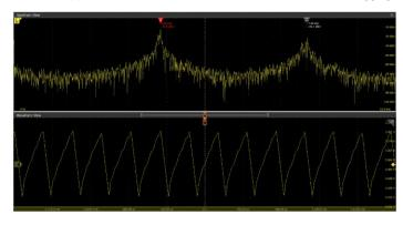
You can analyze cycle-by-cycle by selecting a PWM clock (if available) and view peak-peak and RMS values for each ripple cycle. This gives statistics for all of the cycles within an acquisition. Bandwidth limit capability enables designers to analyze the ripple numbers at different bandwidths.
