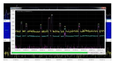
The Time Overview display in application license SMARK provides the +peak (yellow), -peak (purple) and average (blue) traces of the entire recording in a single snapshot. You can use the mouse to identify an area of interest, and this portion of the time record is used to set the start and stop points of the detailed analysis. In this way, you can easily zoom in on active regions, quickly examing areas of interest.
