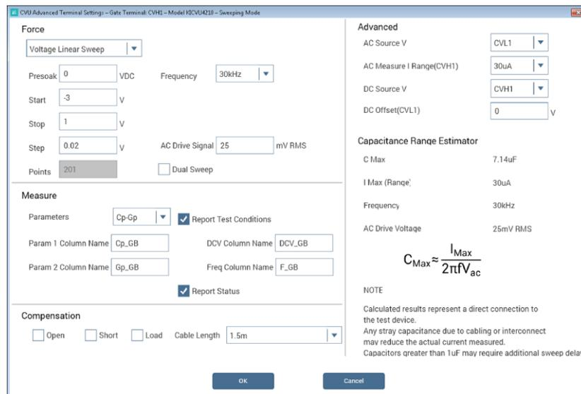
In this test, the CVH1 terminals are internally connected to the AC ammeter and the HI of the DC voltage source by default. The CVH1 terminals are externally connected to the gate of the MOS capacitor. The CVL1 terminals are internally connected to the AC voltage source and the LO of the DC voltage source and are externally connected to the bulk of the MOS capacitor or to the prober chuck.
