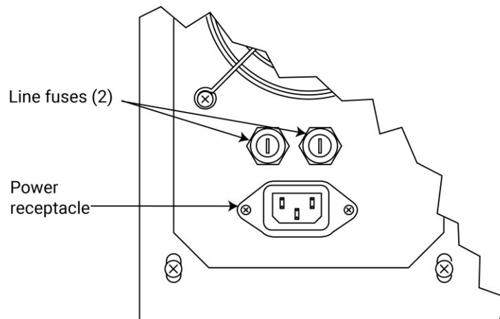
3. Connect the other end of the supplied line cord to a grounded AC line power receptacle.
