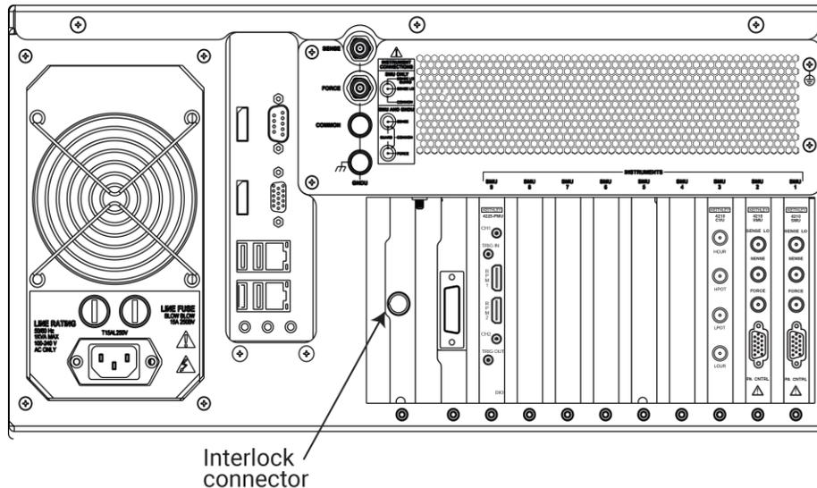
2. Connect the other end of the interlock cable to a compatible test fixture, such as the Keithley Instruments LR:8028.
