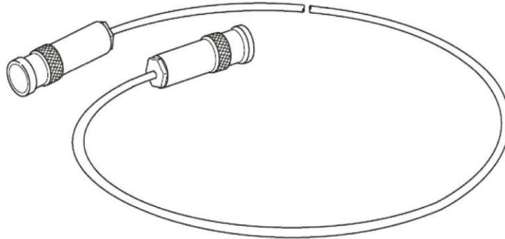
If your system does not have preamplifiers installed, use the cables that have a miniature triaxial connector on one end and a standard 3-slot triaxial connector on the other end. The cable end that is terminated with the miniature connector connects directly to the SMU, and the other end connects to the test fixture or probe station.
