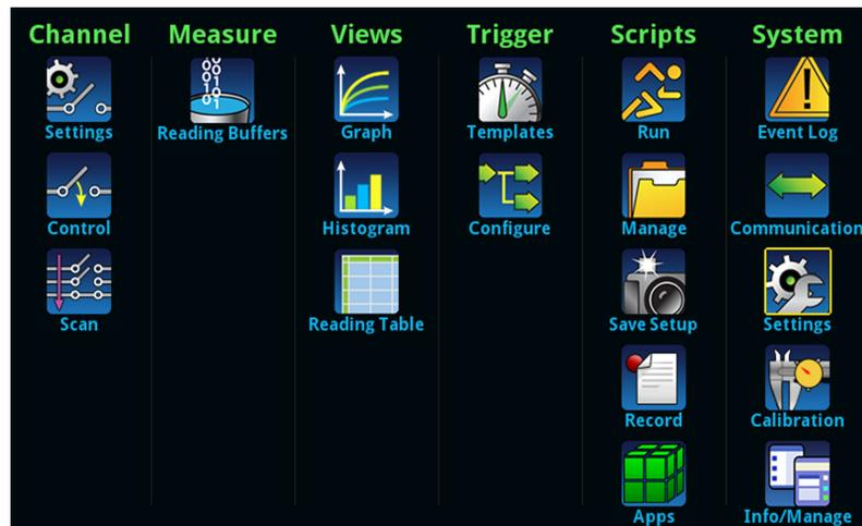
The main menu includes submenus that are labeled in green across the top of the display. Selecting an option in a submenu opens an interactive screen.
