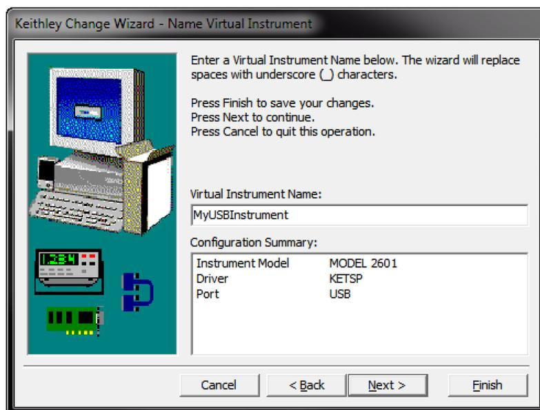
9. In the Virtual Instrument Name box, enter a name that you want to use to refer to the instrument.
