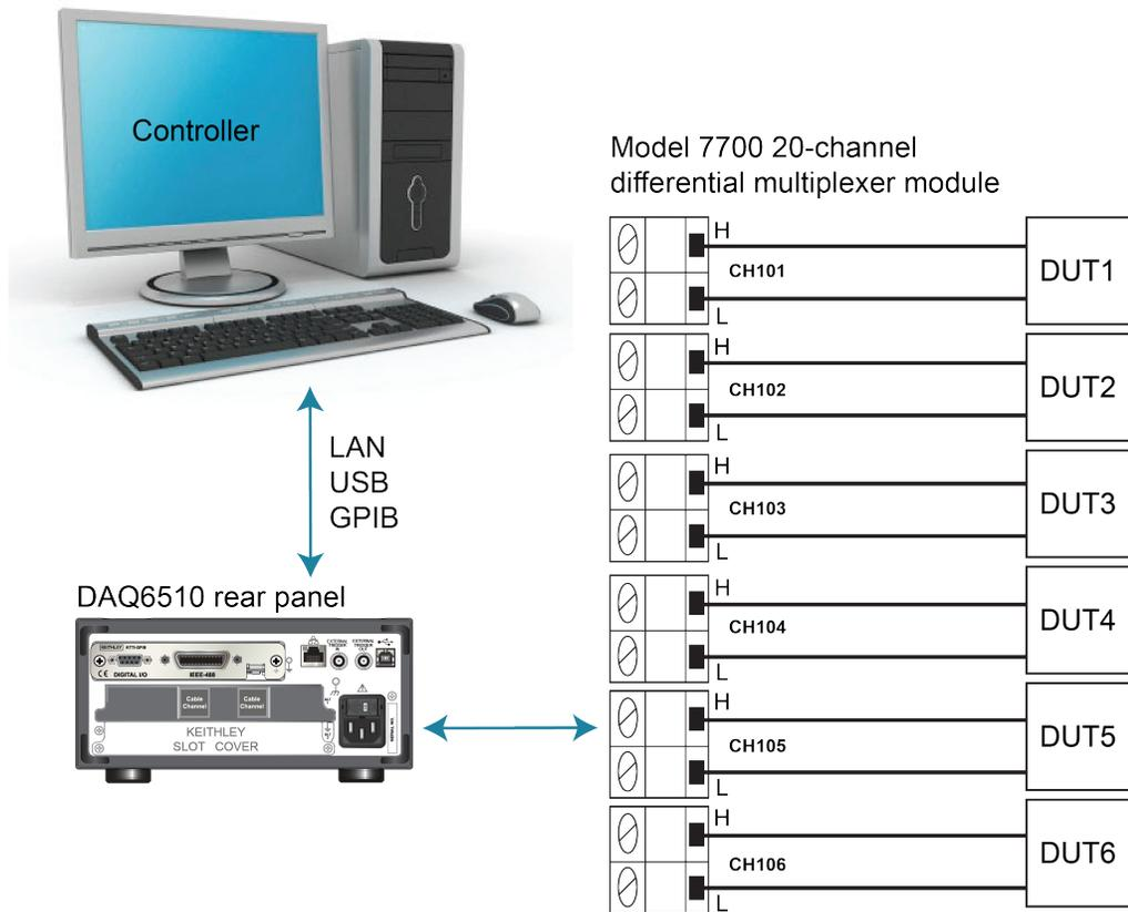
**To connect devices to the instrument:**
