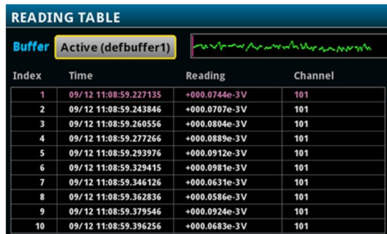
The screenshot shows the 'READING TABLE' interface. At the top, there is a 'Buffer' dropdown menu set to 'Active (defbuffer1)' and a small waveform graph. Below this is a table with four columns: Index, Time, Reading, and Channel. The table contains 10 rows of data, all from channel 101, showing voltage readings in scientific notation over time.
