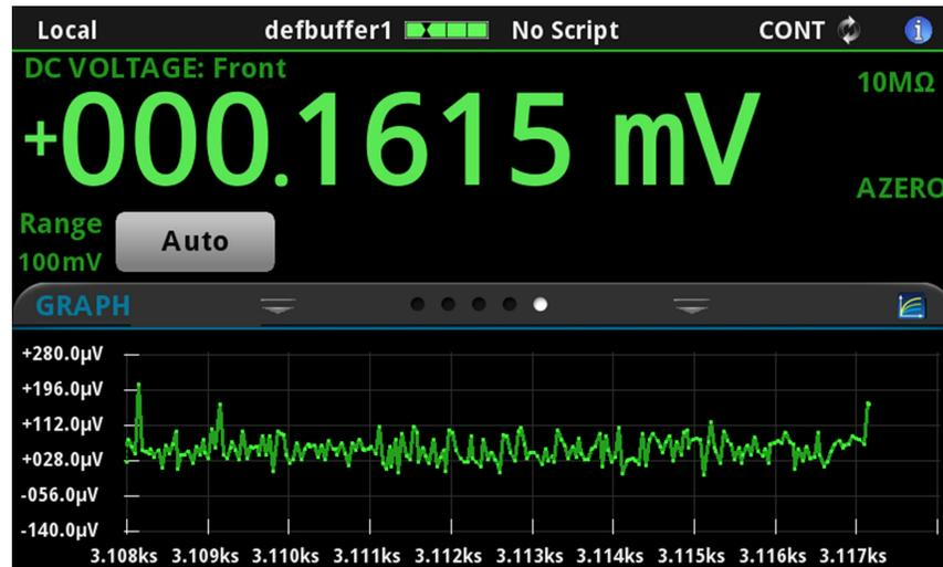
To view the graph in the full screen and to access graph settings, select the graph icon on the right side of the swipe screen header. You can also open the full-function Graph screen by pressing the **MENU** key and selecting **Graph** under Views.
