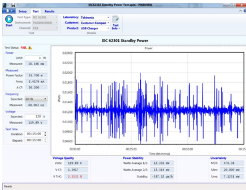
Figure 56: Full compliance IEC 62301 Standby power test
