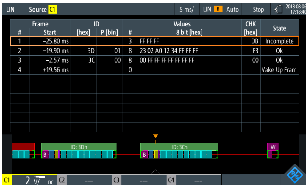
Figure 9-38: Decoded LIN signal in Protocol mode
