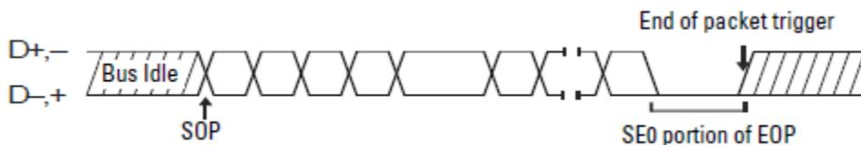
Figure 5-8 USB Data Transmission Protocol
