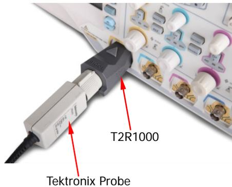
3. Connect the ground terminal of Tek probe to the ground terminal of the circuit. Connect the probe tip of Tek probe to the test point of the circuit under test.
