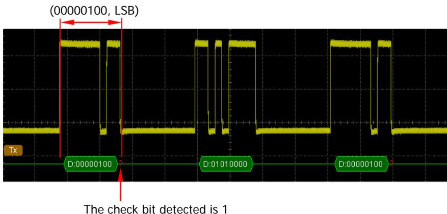
After the decoder is set to none check, the decoding shows no error.
